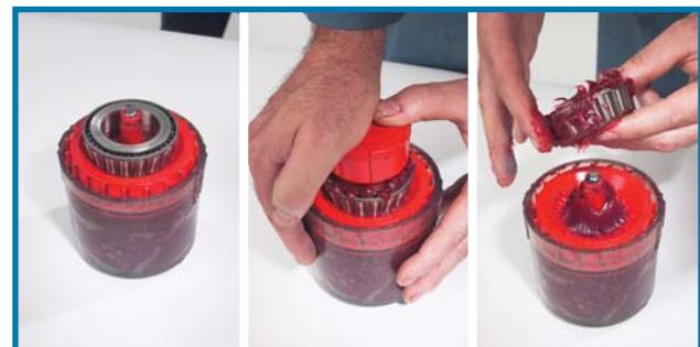
NOTE: For best results, ample space is essential in the housing to allow room for excess grease to be thrown from the bearing and for heat dissipation. It is equally important to retain the grease around the bearing. Normally, the housing should be 1/3 to no more than 1/2 full of grease during bearing assembly. Too much grease in the housing may cause excess churning of the grease and high temperatures.
